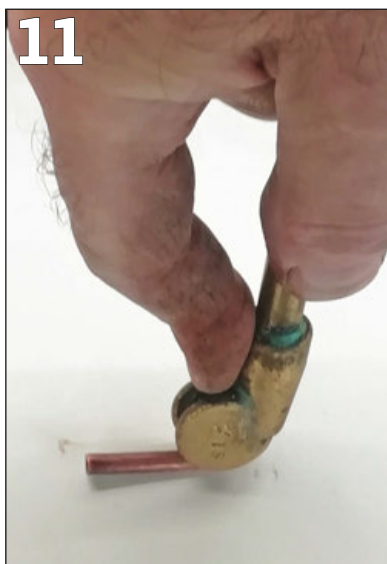
PHOTO 9: \frac{5}{16} -inch pipe wheel bent, crushing on inner radius.
