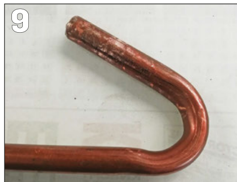
PHOTO 3: The \frac{3}{16} -inch pipe after being bent in the spring.
